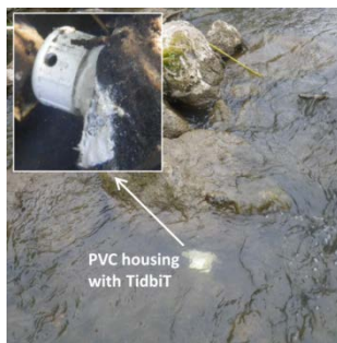
FIGURE 7. PVC HOUSING EPOXIED TO A ROCK.
